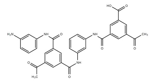
Figure 3. The approximate structure of the aromatic polyamide membrane.
