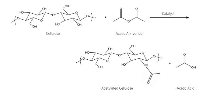
**Figure 1.** When cellulose reacts with acetic anhydride, acetylated cellulose and acetic acid are formed. Commercially available CA membranes are made from acetylated cellulose of varying degrees.
