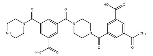
Figure 4. The approximate structure of the piperazine membrane.
