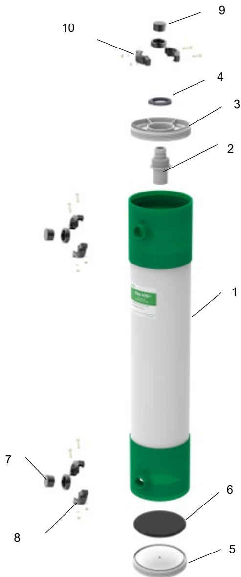
Figure 7. iSep UF module assembly.
