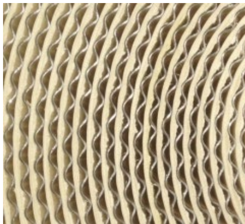
Figure 3. Corrugated flow channel spacer
