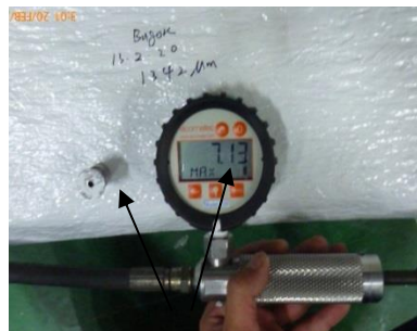
Test of adhesive strength = 7.13 MPa Hydraulic pull off tester (manual)
