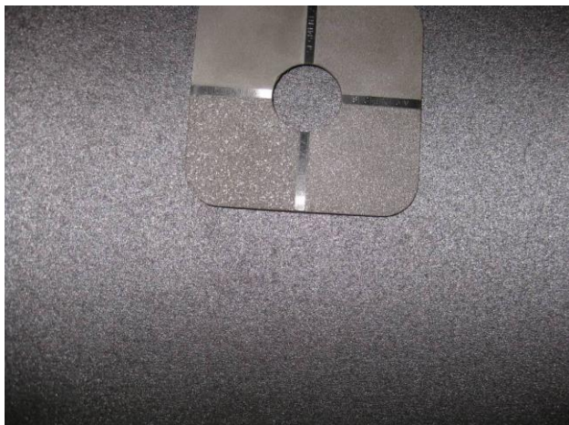
Degree of purity, according to Sa 2½, Rz 40-60 \mu\text{m} ISO 8503-1
