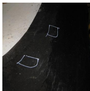
marking the open pores "pinhole"
