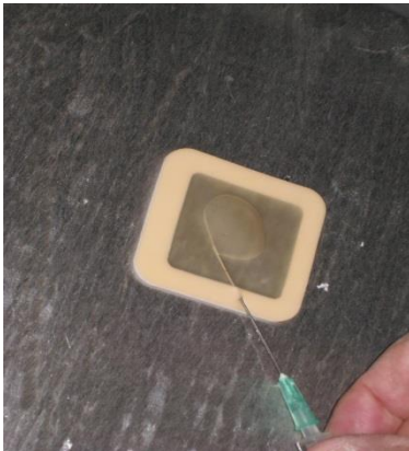
Brestle test sampler with injection of deionized water
