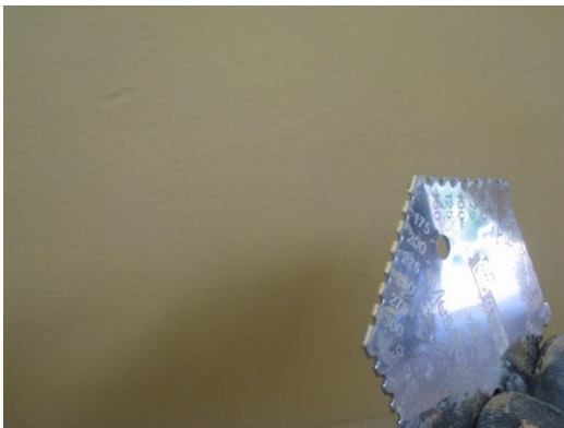
Wet film comb, film thickness measurement (stainless steel comb)
