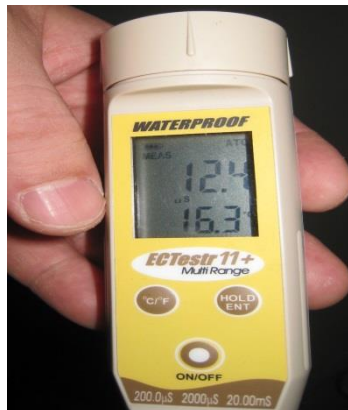
conductivity meter measurement result: 12.4 mg/m 2 (NaCl)
