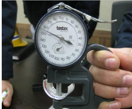
roughness measurement of blasted surfaces "Testex Press-O-Film Kit"
