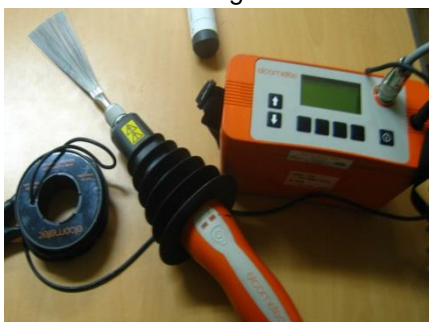
100% pore examination of coating, according to ISO 2746 (ASTM D 5162)
