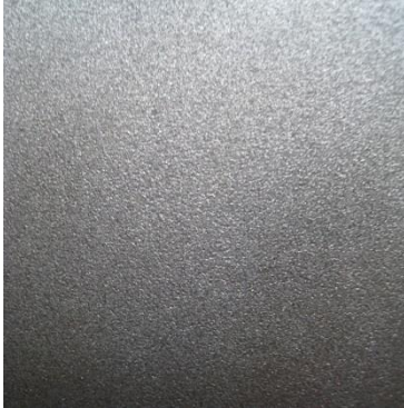
Blast profile of the surface after Sa 2½, Rz 40-60 µm
