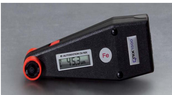
Dry film thickness measurement by means of a digital LCD Qnix®1500 measuring device
