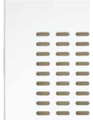
Tangent, 4 x 14 mm, 10/20 mm c/c Perforation: 21.3%
