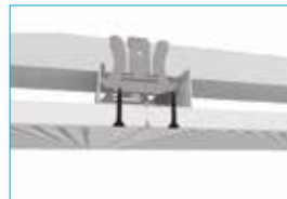
Edge B (bevelled edge) Visible joints For Globe
