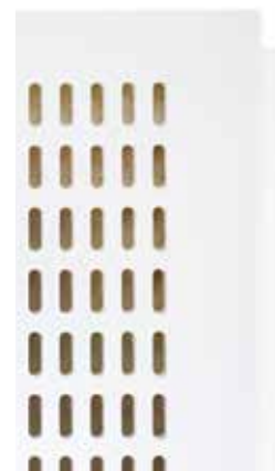
Tangent, 4 x 14 mm 10/20 mm c/c Perforation: 21.6%
