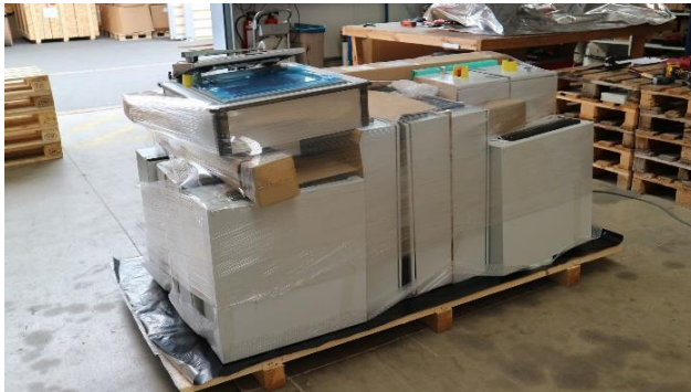
Example: Fixture for supporting the packaged goods
