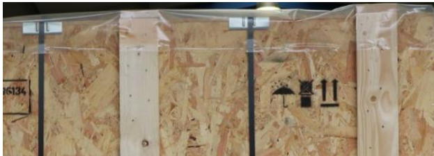
Example: Edge protection outside
