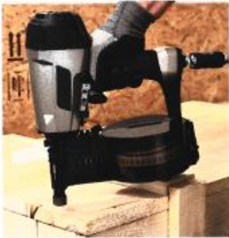
Driving in of fasteners with the pneumatic nailer
