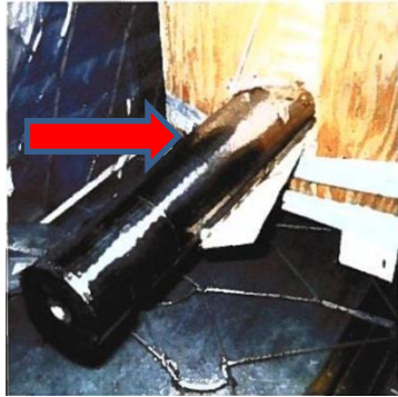
Example: Acceleration forces are often underestimated. Here, a not properly secured cylinder will break through the packing case wall. Source: HPE
