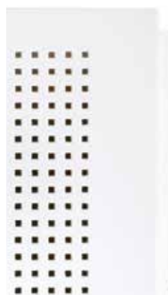
Micro, 3 x 3 mm 8,3 mm c/c Perforering: 10,6%
