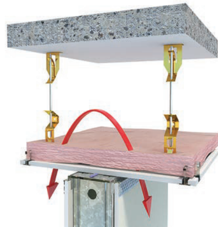
Figure A4: Sound Transfer Over Partition
