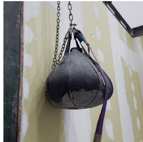
Figure A14: Large Soft Body Impact Testing
