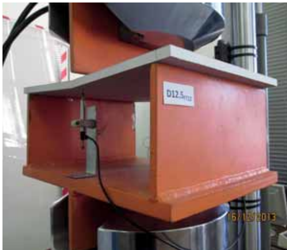
Fig. 4.53: Bending tests on cladding panels
