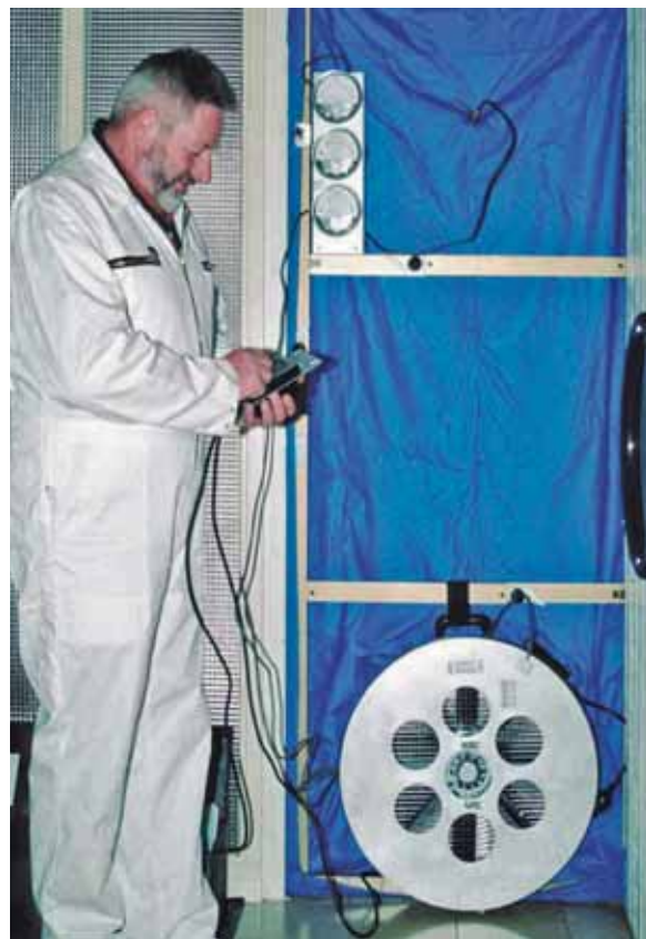
Fig. 6.26: Blower door measurement for determination of the air exchange rate n_{50} /Knauf Gips KG/
