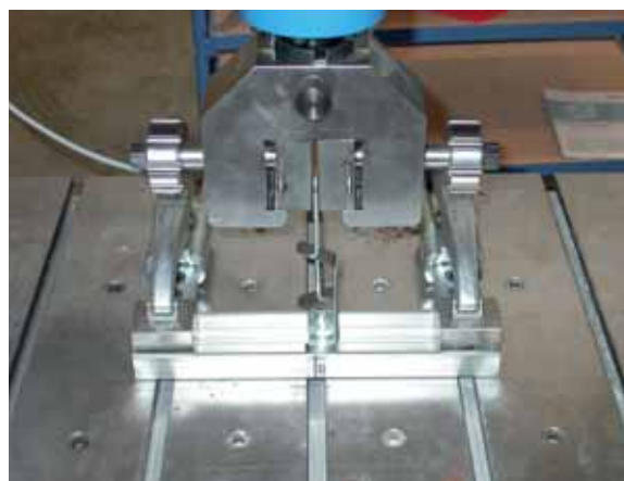
Fig. 4.22: Tensile test on a suspender in conjunction with a carrying channel section
