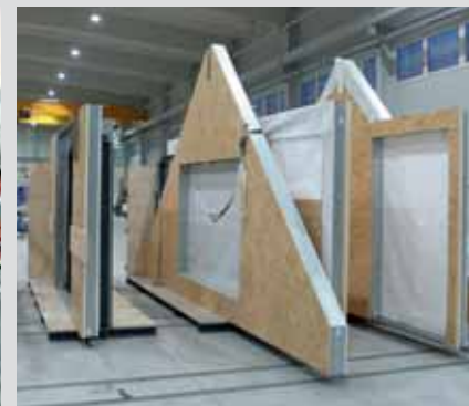
c) Cladding-braced solution /Cocoon/
