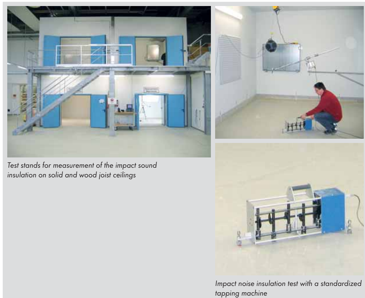
Fig. 6.6: Building acoustic test stand of Knauf Gips KG for measurement of the impact noise insulation using a standardized tapping machine /Knauf Gips KG/
