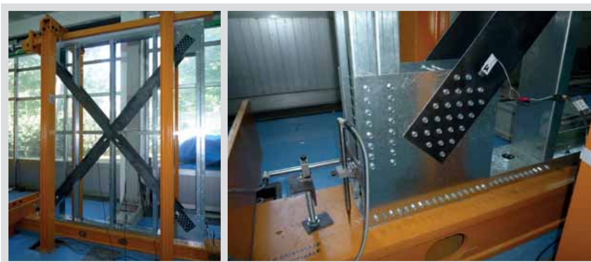
Fig. 5.27: WHD general view and corner detail
