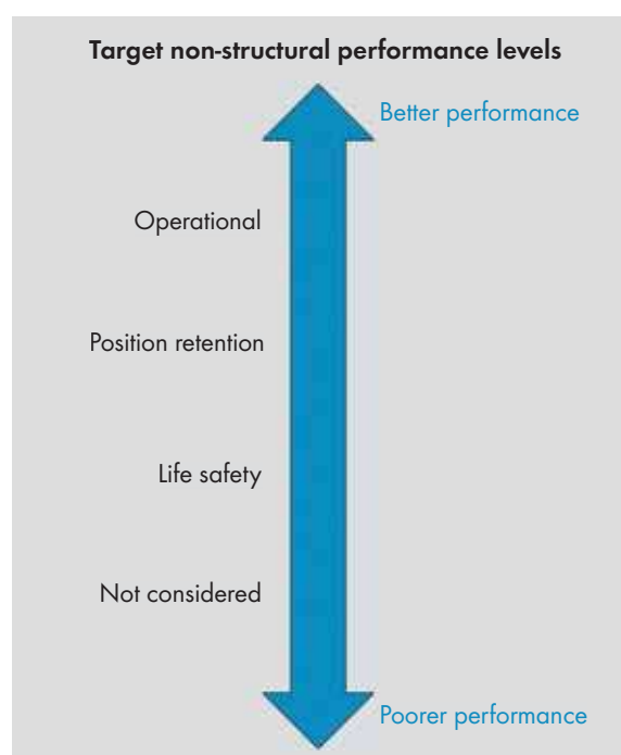
Fig. 4.39: Target non-structural performance levels
