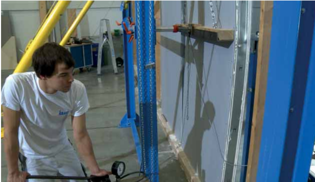
Fig. 4.19: Line load test used for applying static loads to partition walls
