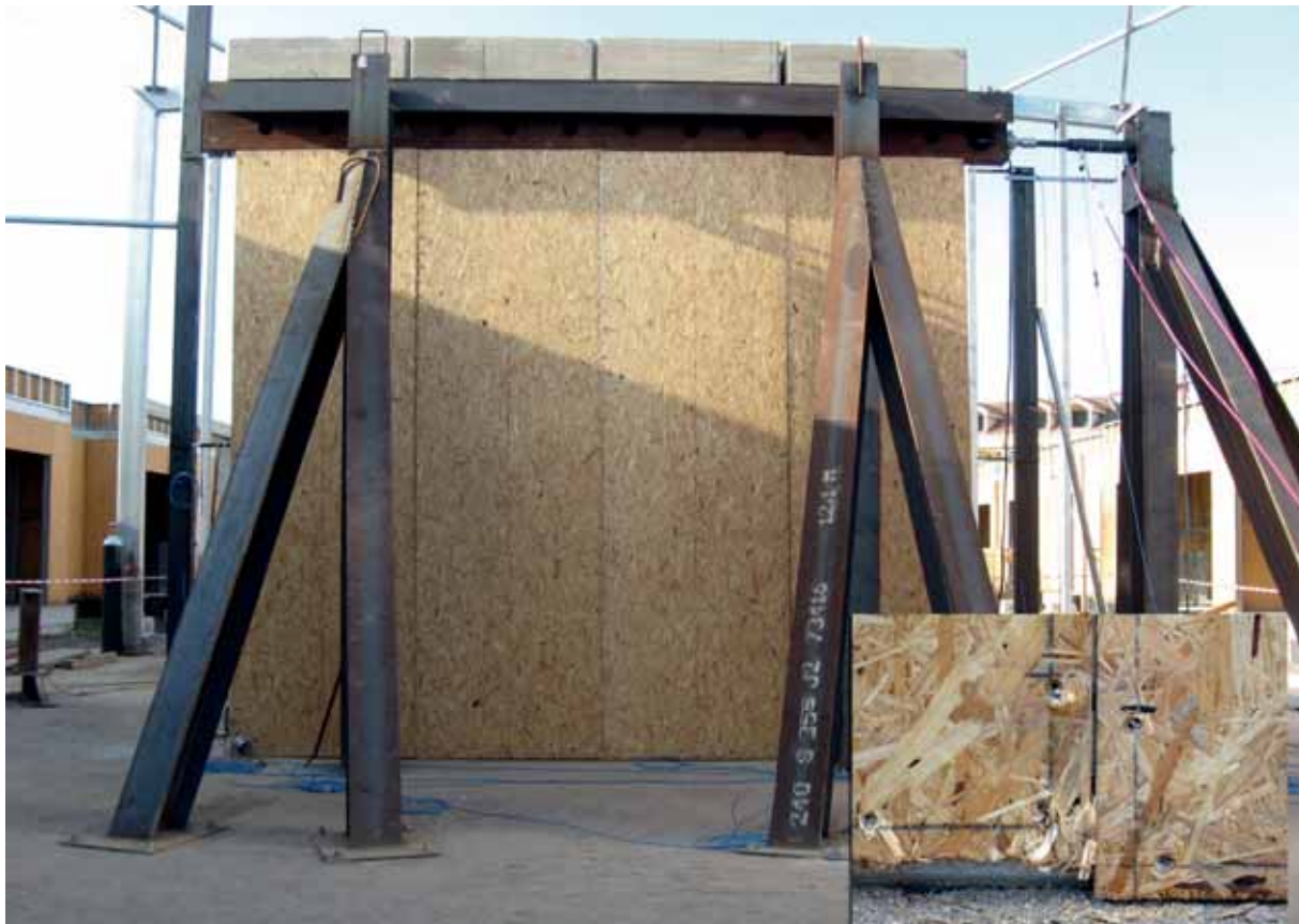
Fig. 5.60: Shear test on walls
