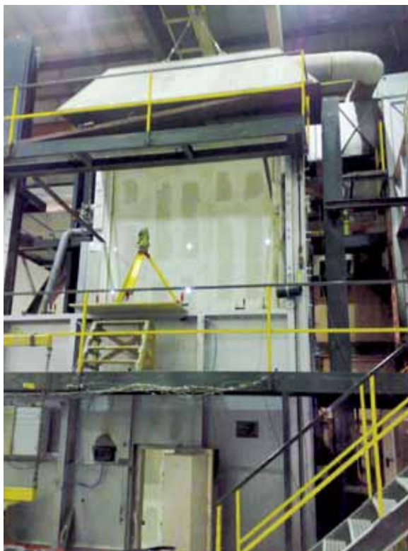
Fig. 6.2: Test of a 7 m high partition to F90 at the MPA Braunschweig /Knauf Gips KG/
