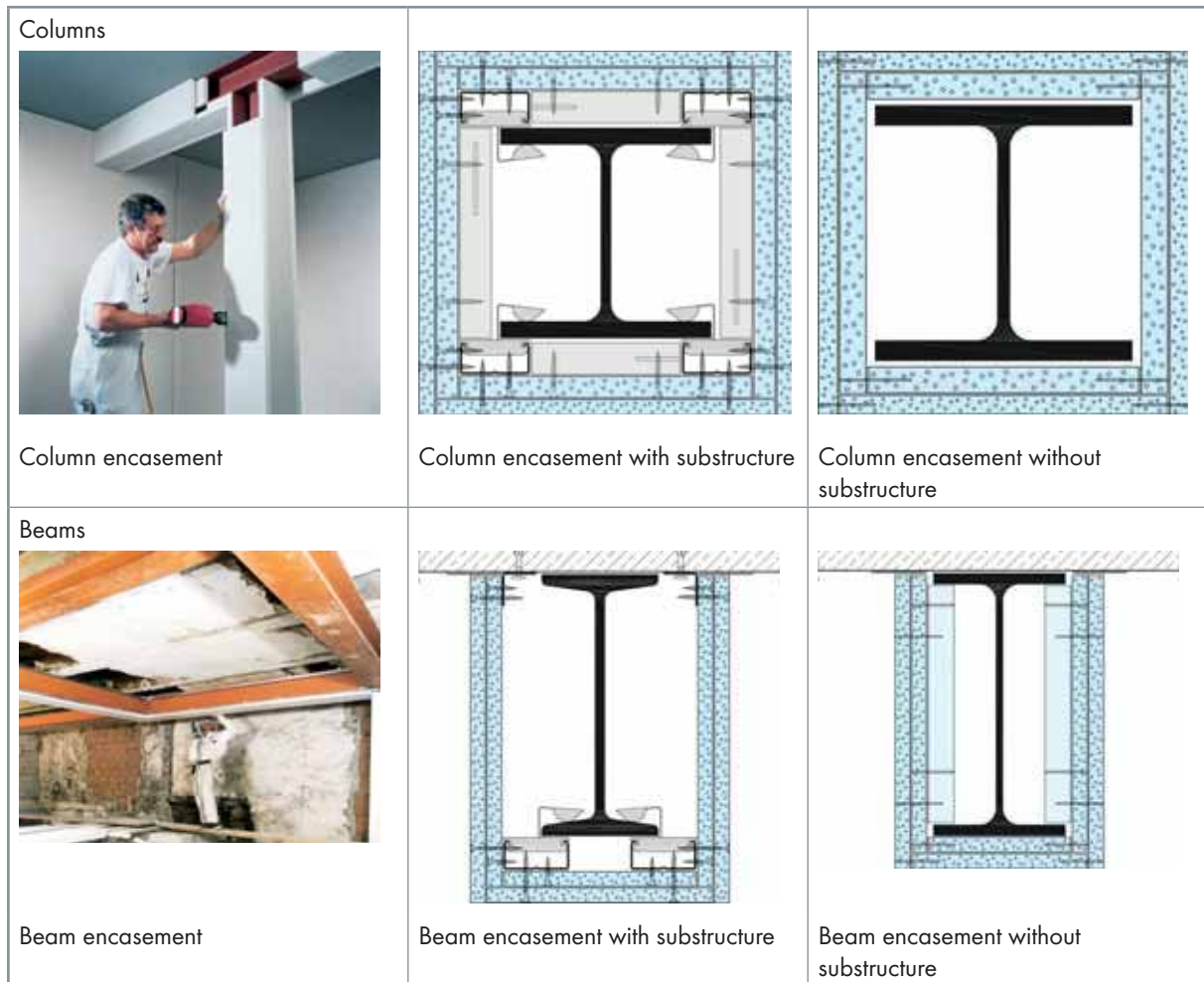
Fig. 3.23: Application examples of columns and beams in comparisons with and without a grid using Fireboard and double layer cladding /Knauf Gips KG/
