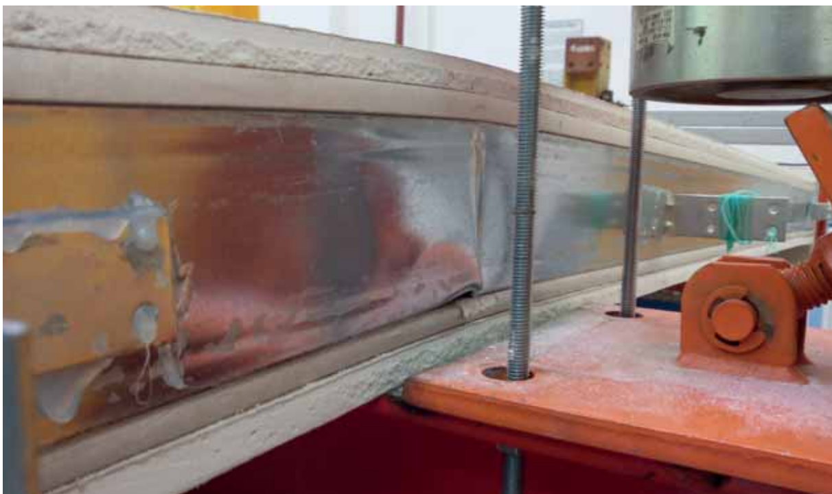
Fig. 4.61: Typical failure mode of out-of-plane monotonic tests
