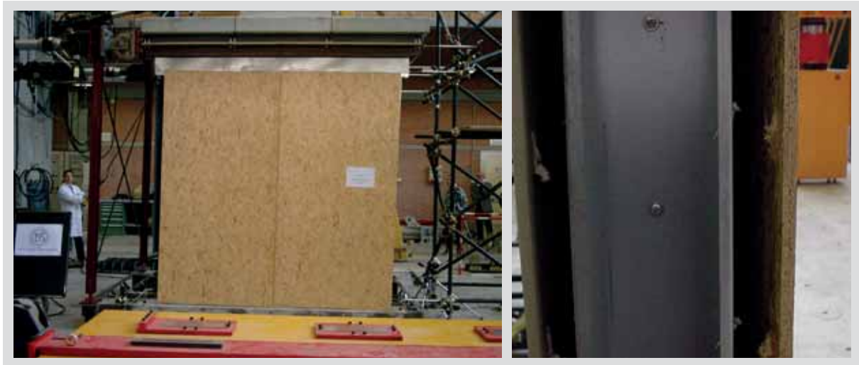
Fig. 5.23: Global collapse mechanism of a wall due to failure of cladding-to-frame connections
