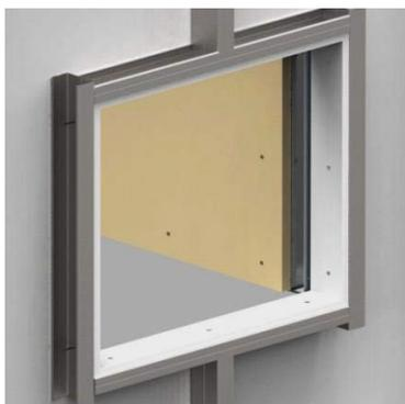
EN - Cover the inside of the CW profiles all around with plasterboard strips starting from 500x500mm and upwards. The distance between the insulation of the door and the plasterboard strips is  $\leq 5$  mm, the distance between the screws is  $\leq 200$  mm.
