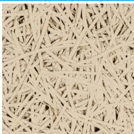
HERADESIGN® Fine is a Cradle to Cradle Certified® Gold\*, acoustic ceiling and wall panel made from single layer, magnesite bonded wood wool (fibre width 2mm).
