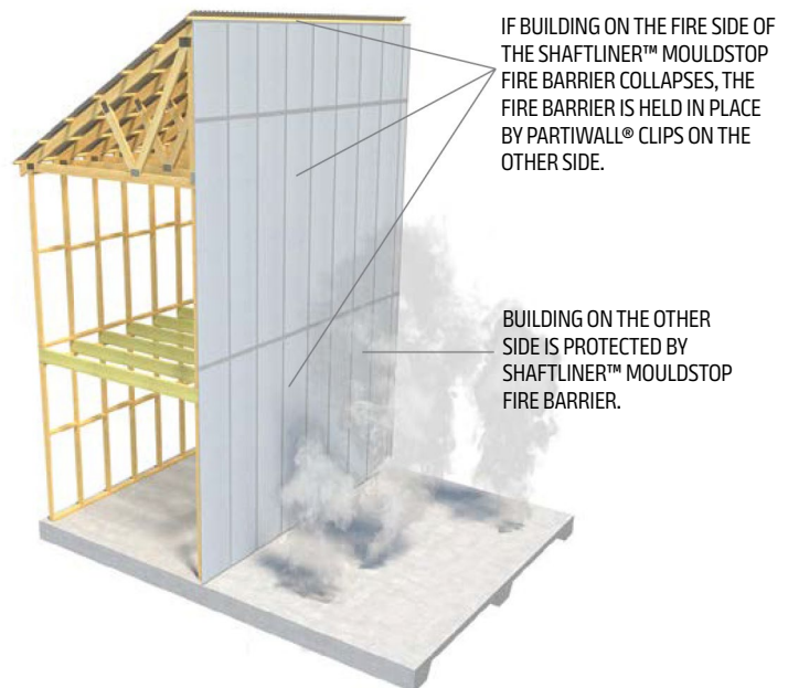
Figure 2.3: After the fire
