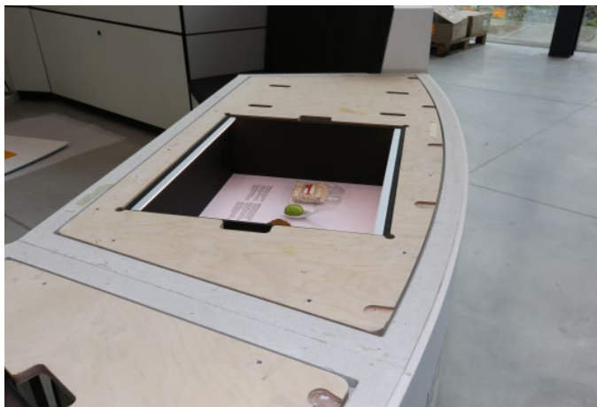
The exhibition display cabinet is fitted to the precision milled module. A glass cover and white table top will round off this module.
