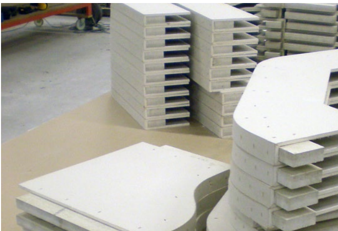
Finned section during prefabrication: The prefabricated side elements of the fins are backed by 18 mm thick gypsum fibre boards.
