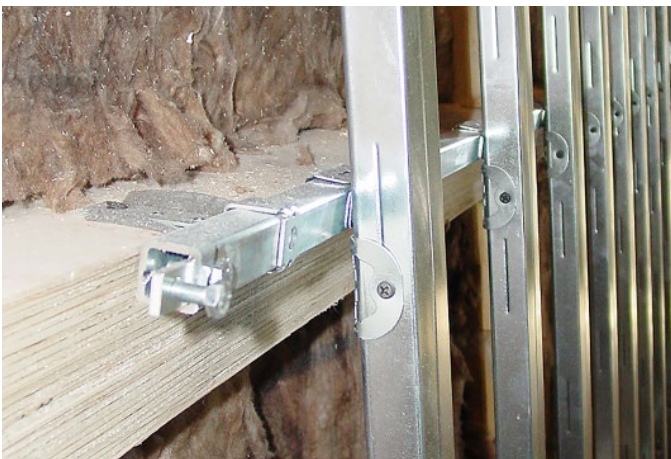
A detailed look: Curved CD channel 60/27, curved horizontal square tubing 20x20x2 with CD profile connectors and suspenders for square tubing on felt separating layers. (Photo: Knauf)
