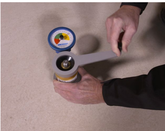
Figure 79: Test of the bond strength
