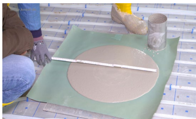
Figure 56: Measurement of the diameter
