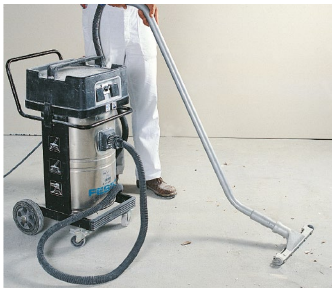
Figure 29: Cleaning with an industrial vacuum cleaner
