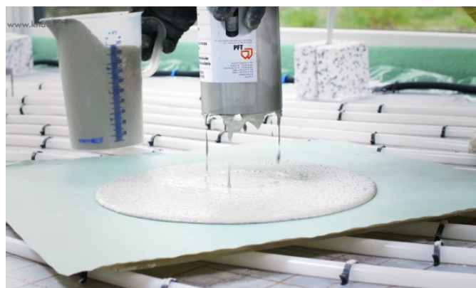
Figure 55: Lift the consistence checking tin
