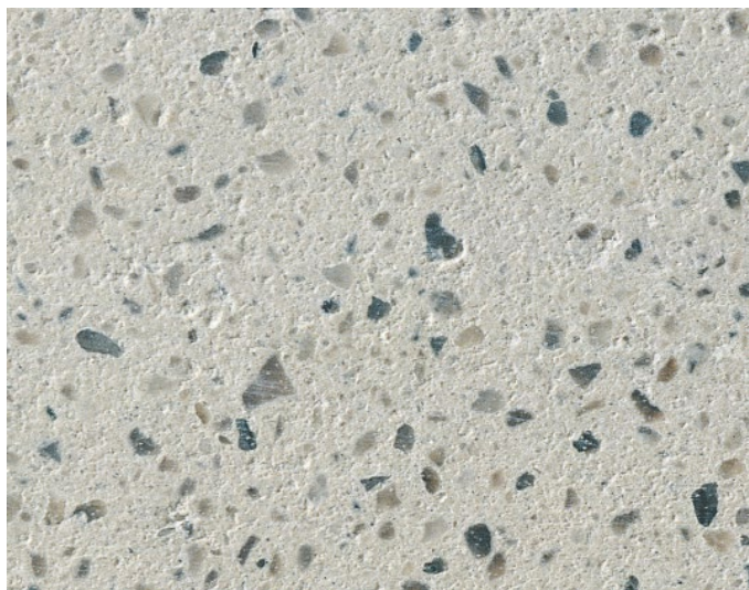
Figure 75: Knauf flowing screed cross-section, magnified by 4
