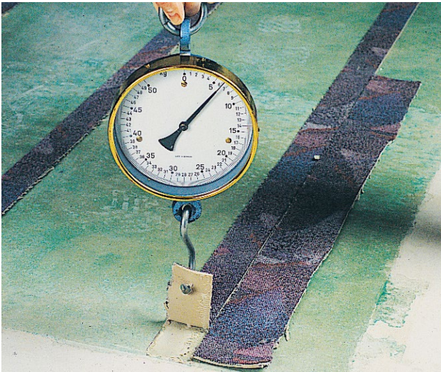
Figure 78: Bonding test and test of the resistance to peeling
