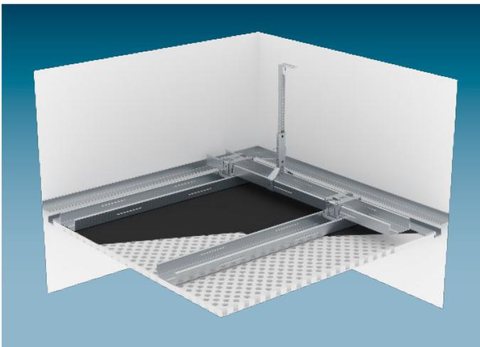
Cleaneo UFF plaster base boards with fleece or foil lamination on the rear side are screw fastened to a metal grid of carrying and furring channels (double-layer profiles) made of sheet metal profiles CD 60/27. Anchoring of the CD channels is undertaken with suspenders on the basic ceiling. An acoustically effective insulation layer can be laid upon the furring channels.
