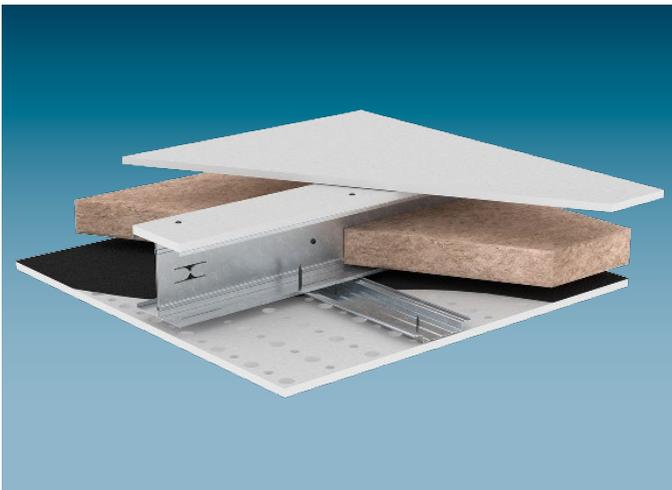
Cleaneo Classic boards are fixed with screws to a metal grid of carrying channels made of double profiles types CW or UA with covering strips as well as furring channels made from hat-shaped channels. The carrying channels are anchored only to the flanking walls.
