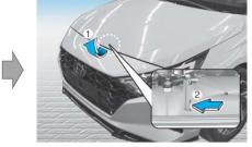
Raise the hood slightly, push the secondary latch up (1) inside of the hood center and lift the hood (2)
