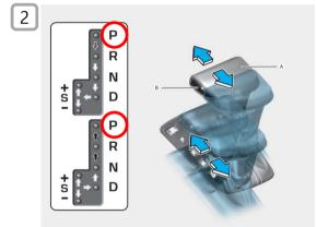
If automatic transmission: move shift lever to parking position (P)
