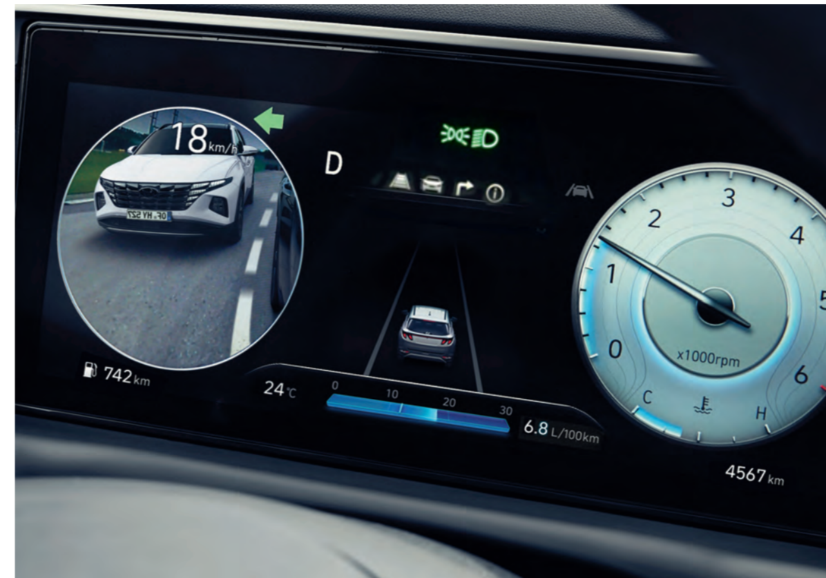
Blind Spot View Monitor (BVM) Making tricky lane changes safe and easy. Now you can see the rearward left- and right-hand side views on a screen in the digital cluster. The cameras are activated by the use of the turn indicator.
