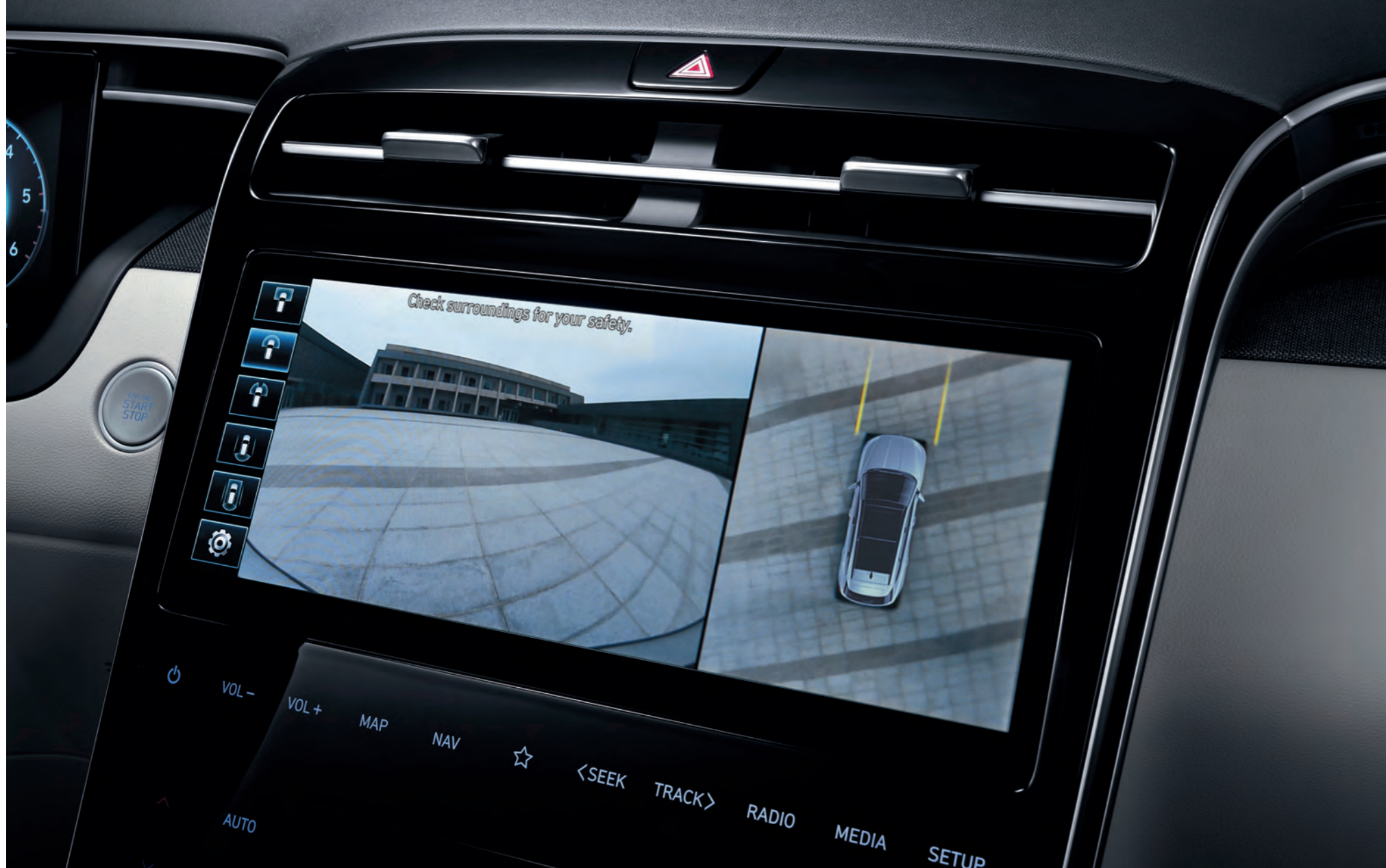
Surround View Monitor (SVM) Enjoy 360° visibility for easier and safer parking. Four high definition cameras mounted on the front, sides, and rear of the vehicle show the surroundings in real time.
