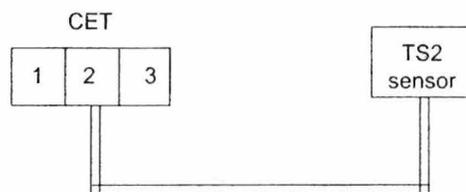
Cable Specification : minimum cross section 0.5mm<sup>2</sup>
