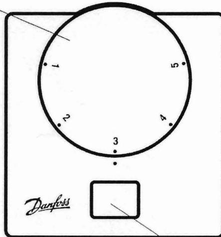
LCD Display. During normal operation cylinder temperature is displayed. When setting dial is moved the display momentarily changes to show set temperature.
