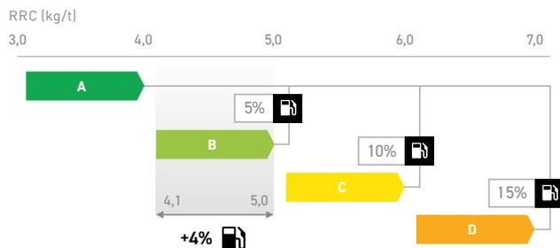
*Relationship between tyre RRC grade and vehicle fuel consumption. Results based on VECTO's long haul cycle for default tractor/trailer combination.*
