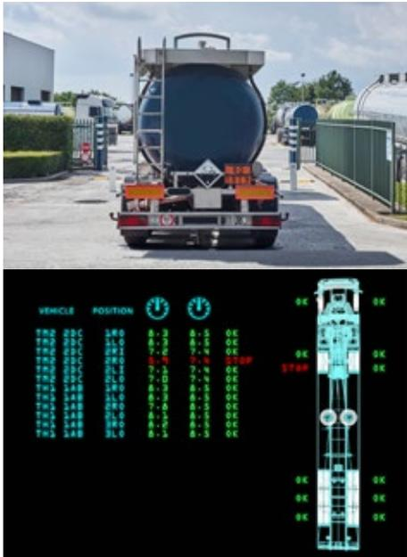
With Tirematics we go a step further with pro-active tyre maintenance through an automated inspection system.
