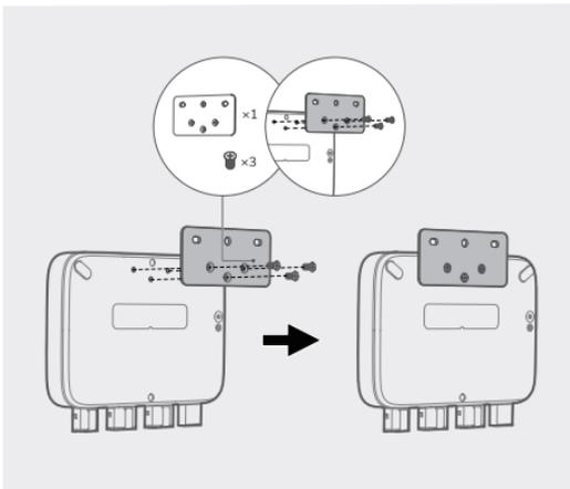
3. Insert ST5.5\*25 into M5\*40 through holes of the board.
