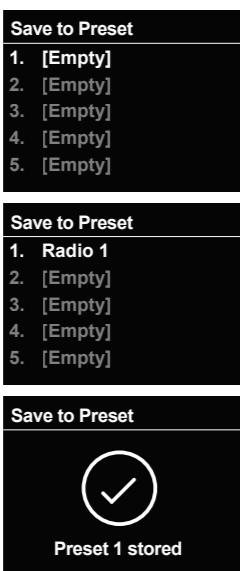
To save the current playing radio station to a quick preset button, simply hold down the desired preset button for 2 seconds.
