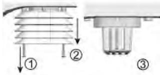
5. Unscrew the 2 screws at the bottom of the radiation shield.
