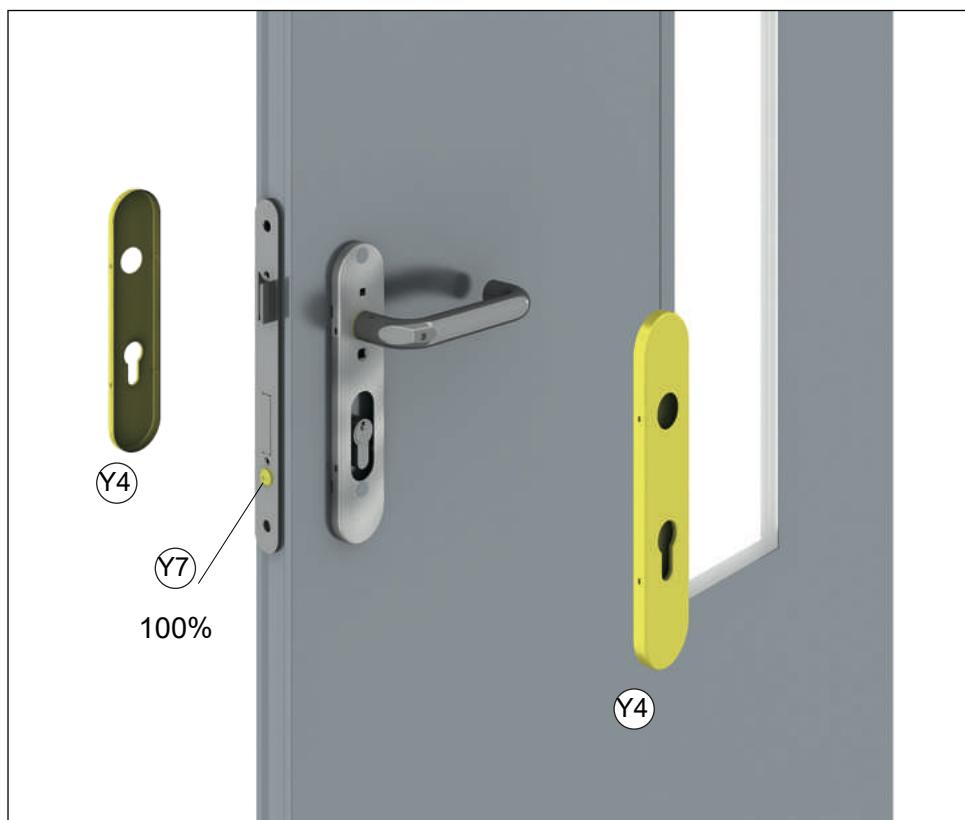
The Bolts (Y7) should be fully tightened
