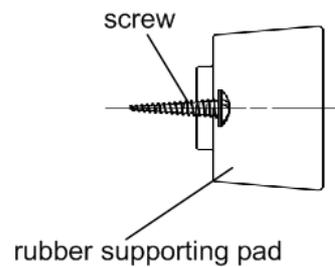
3. Make screw in alignment with the hole on lower base cover. Fasten rubber supporting pad to the base cover firmly by a cross screwdriver (self-provided).
