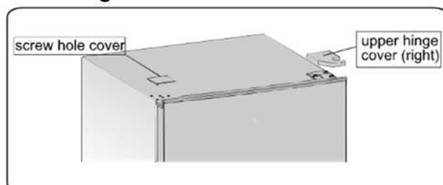
2. Unscrew the special flange self-tapping screws which are used for fixing the right upper hinge part by an 8mm socket driver or a spanner (please
