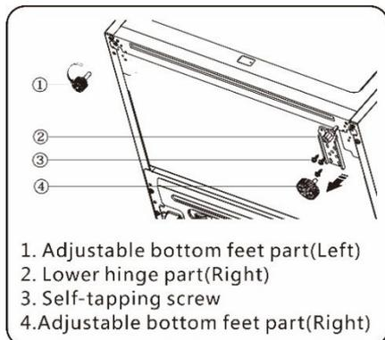
6. Loose out the lower hinge pin, change it to the reverse hole site, then tighten it into position follow the picture below.
