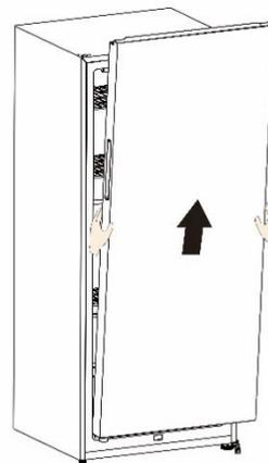
4. Place it on a smooth surface with its panel upwards. Loose screw 2 and part 1, then install them to the left side and tighten securely.
