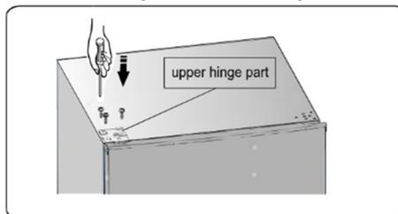
10. Install the big screw hole cover (which is in the plastic bag) on the top right corner of the refrigerator. Install the upper hinge cover (which is in the plastic bag) on the left corner. Put the other upper hinge cover into the plastic bag.
