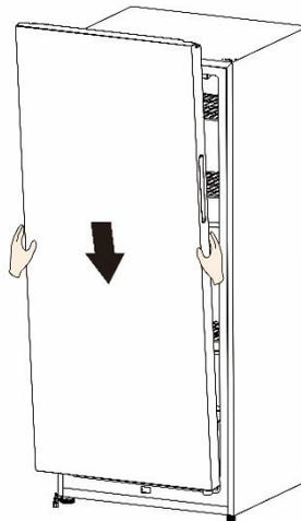
9. Transfer the upper hinge part and make the upper hinge axis into the upper hole of the door, and adjust the position of the door (please support the door with your hand when doing it), fixing the upper hinge part with the special flange self-tapping screws.
