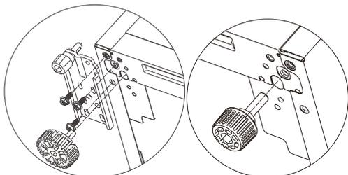
8. Transfer the door to the property position, adjust the lower hinge part, and make the hinge axis into the lower hole of the door.
