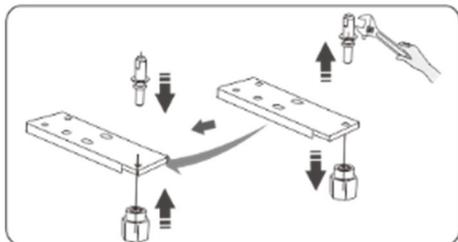
7. Replace the lower hinge part to the left side and fixing it with the special flange self-tapping screws. Replace the adjustable bottom feet parts to another side and fixing it.
