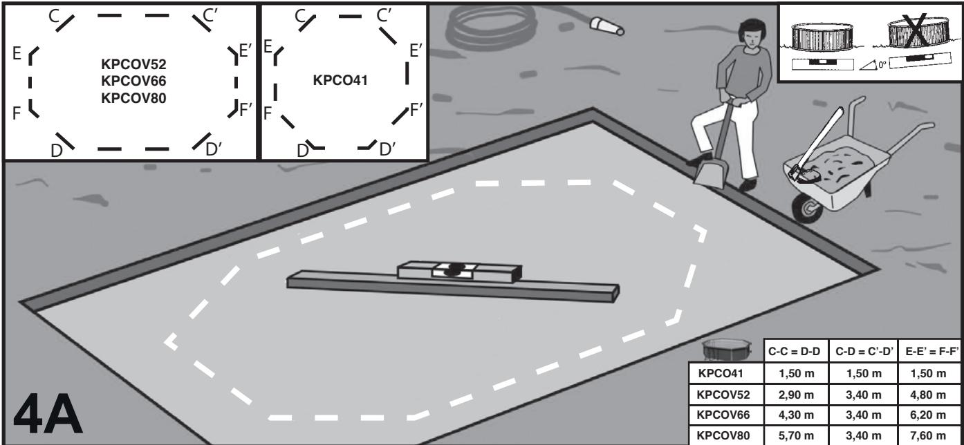
**EN OPTION 4A: INSTALLATION OF THE POOL ON THE GROUND - Levelling:** When levelling the ground, always remove material from the top of the slope rather than filling in the bottom: this will ensure greater ground stability and firmness. Always remove all grass, roots, stones, etc. Levelling is extremely important: devoting the necessary time and effort to ensuring that your pool sits properly on the ground will avoid problems later.
