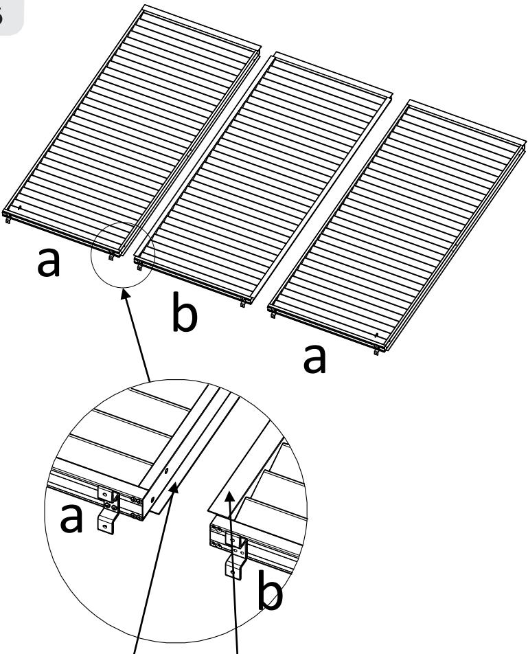
**When assembling the shutter walls, note the side tube direction:**
