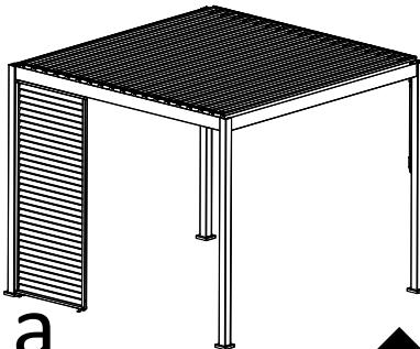
**Adjust the spacing to ensure that the three shutter walls are roughly equally spaced.**
