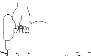
If the floor is a wood floor, you don't need to knock in the plastic expansion pipe, directly use J to knock in the floor.
