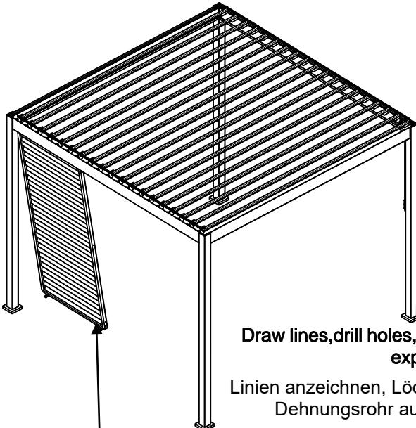
**Draw lines,drill holes,tap in plastic expansion pipe.**
