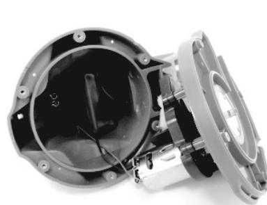
3. Remove the battery pack to expose the PCBA. To detach the battery connection wire, press the clip on the connector and then pull it out. **NOTE:** Wrap the connector immediately with insulating tape in order to avoid short circuit caused by contact of both wire terminals.
