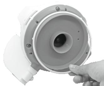
2. Use the screwdriver to unscrew the 4 screws located on the bottom of the head to release the bottom plate at first. Use the screwdriver to unscrew all the screws on the base as shown. Remove the impeller and then pry up the base and remove it to expose head inside.
