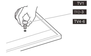
You are provided with 4 diameters of TV fixing screws, **M4**, **M6** and **M8**. Determine the screw diameter that fits.
