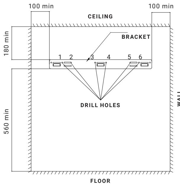
**2.1C** Insert the wall plugs into the drilled holes and use the six ST5 x 40 screws to fix the mount to the wall.
