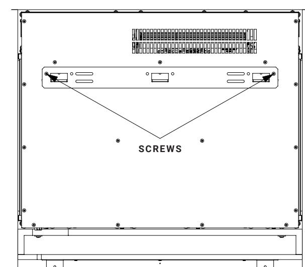
**2.1B** Choose a stable wall and mark the six holes of the wall mount. Drill the marked holes using the appropriate drill bit.
