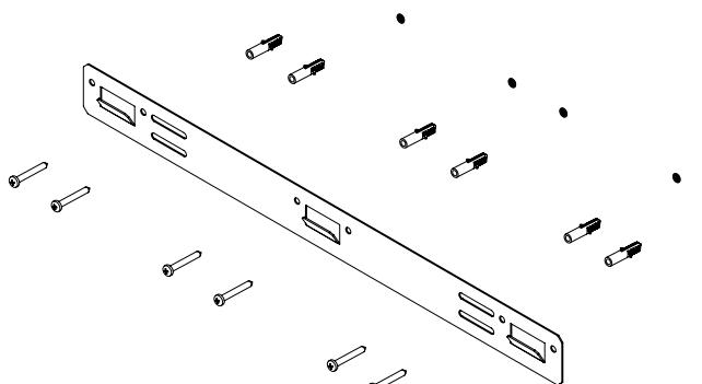
**2.1D** Hang the electric fireplace on the wall mount and mark the two holes on the L-supports which are attached to the lower part of the fireplace. Then take down the fireplace.
