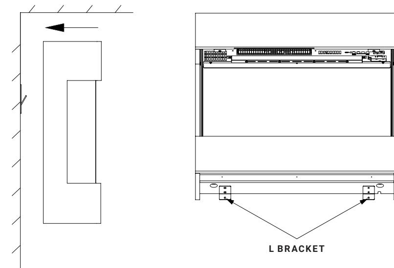
**2.1E** Drill the two holes with an 8 mm drill bit and insert the wall plugs. Hang up the electric fireplace again and use the two screws ST5 x 40 to attach the L-support to the wall.
