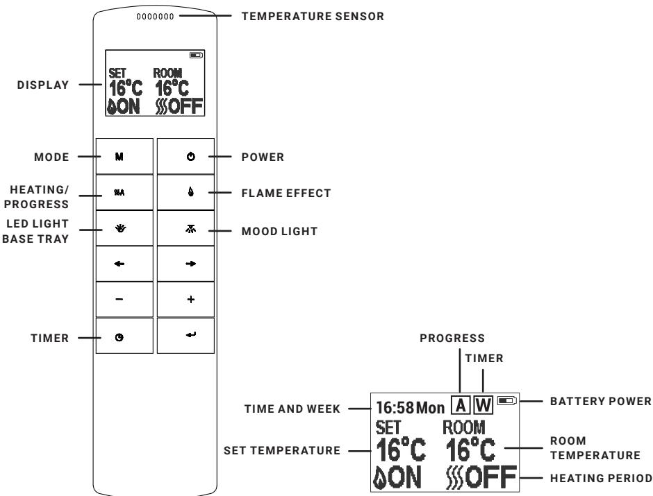
**NOTE:** This is a thermostatic remote control. The remote control should be in the same room as the fireplace and lie on a flat surface. The remote control must be placed away from the fireplace so that hot air does not affect the thermostatic reading.
