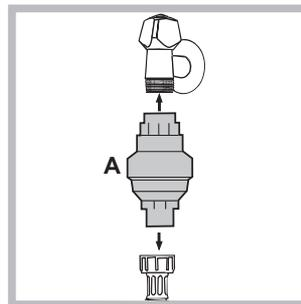
1. Screw the device "Water Block" (A) to a cold water tap with the threaded connection and then screw the water hose to the device.
