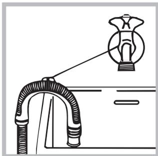
! We advise against the use of hose extensions; if it is absolutely necessary, the extension must have the same diameter as the original hose and must not exceed 150 cm in length.
