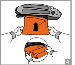
5. Now push the airbags in the designated compartments. The suction and release valve must be clearly visible on top of the airbag material.
