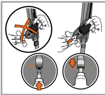
Only then is the handle attached properly and ready to use. Dose the coupler with a drop of ABS oil at regular intervals so that the handle can be attached and detached easily. This prevents accidental activations. If the handle will not attach refer to point 13.1. If the handle is not attached properly and
