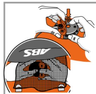
Now fold up the red cover and press the release valve in the center of the black suction and release valve. At the same time, compress the airbag until it is completely empty.
