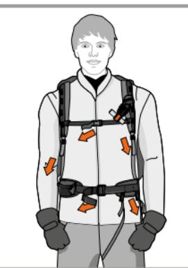
The carrying system meets the high European standards (TÜV guidelines) for extreme operational demands. The tensile strength for all weight bearing straps equals 3000 N (674lbs).
