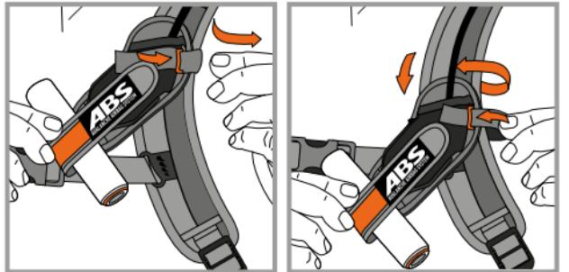
and unfold the Velcro fastener, detach the plastic grommet and thread it through the little straps one position up or down. Reattach the handle plate to the newly positioned grommet and reattach and secure the Velcro fastener.
