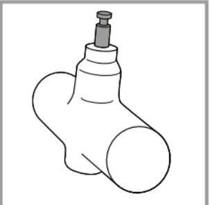
**The pin has to be firmly fixed and the red line should not be visible. If the red line is visible on the pin, the handle has not been charged and therefore will not function properly!**
