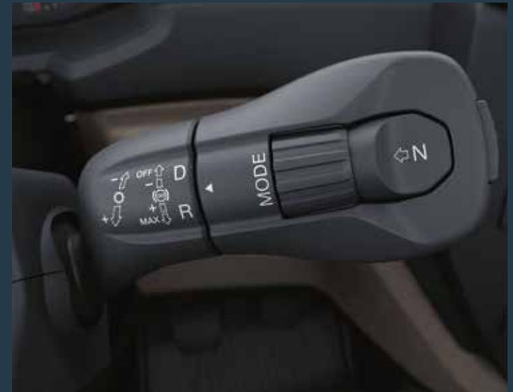
Operation of the gearbox using the right control stalk is a completely new development. Both driving mode and driving program are selected by means of the stalk switch. Controls located in easy reach near the steering wheel and electric parking brake make for certainty in operation.
