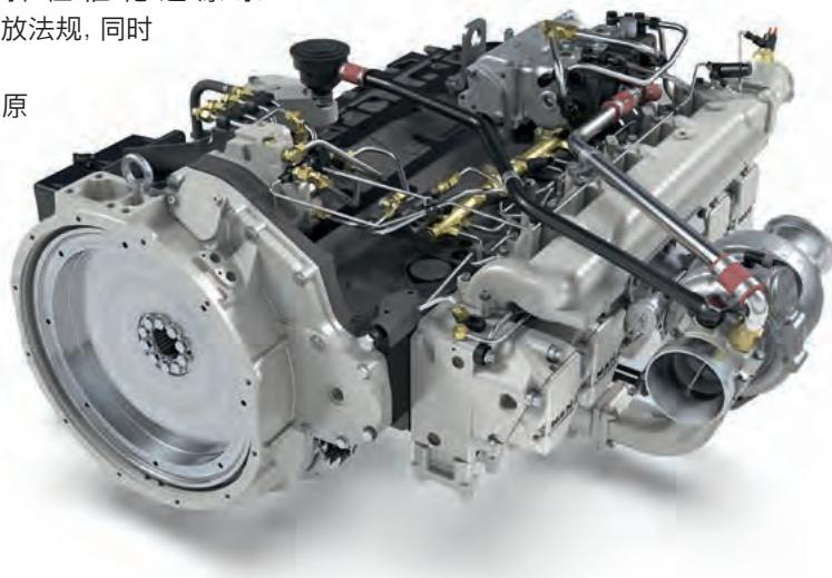
MAN engines are fitted with an exhaust-gas aftertreatment system in accordance with the SCR process: in this way they comply with the emission levels required by 04/26 EU Stage 3B but still achieve high efficiency and low fuel consumption figures. SCR (Selective Catalytic Reduction) is a chemical process that removes oxygen with the aid of a reducing agent, thus (selectively) reducing the nitrogen oxides in the exhaust gas.
