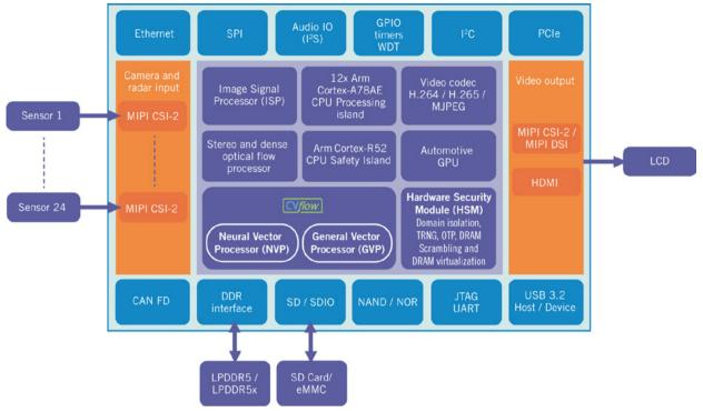
FIGURE 4 Block diagram of the CV3-AD685 SoC (© Ambarella)
