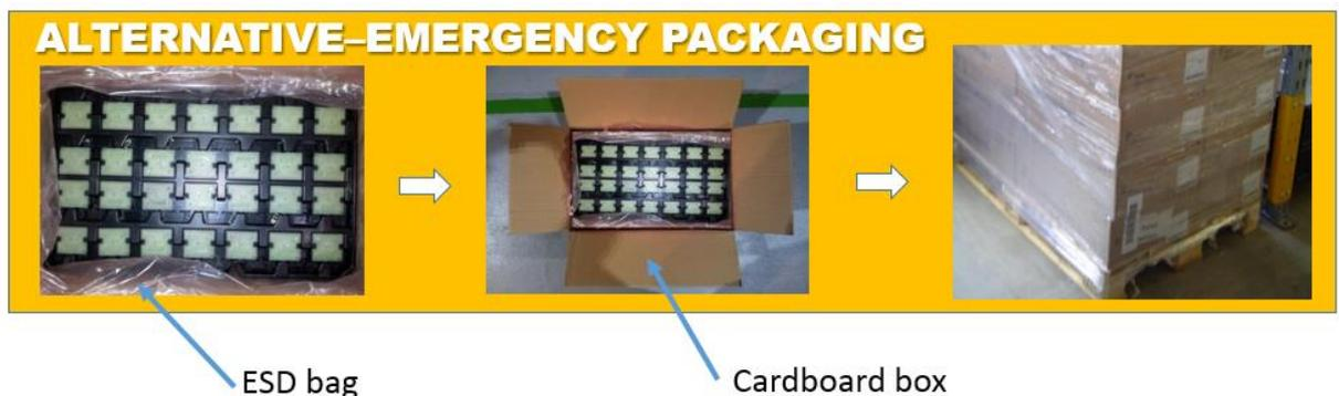
Figure 5.4-2: Example of alternative non ESD cardboard box (with ESD plastic tray and ESD bag)
