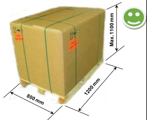
Figure 5.1-2: Not acceptable (left) and acceptable (right) loading units (LU)
