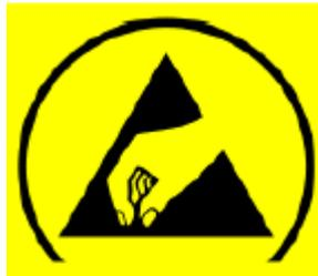
Figure 5.5-1: Example of ESD protection marking
