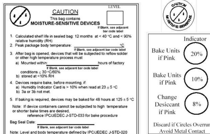
Figure 6.2.5.2-2: Indicator Card (HIC), “Moisture-Sensitive Identification” (MSID) and Moisture-Sensitive Identification Label “Caution-Label”
