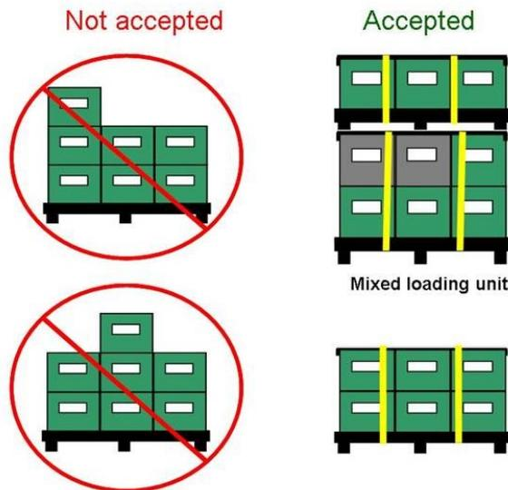
Figure 9.2.3-2: Not acceptable and acceptable LU with small load carrier
