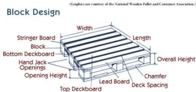
Figure 8.1-1: Definition of a 4-way-free-entry block pallet
