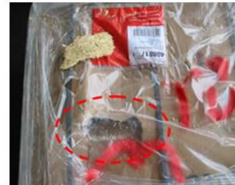
Damaged carton cover by foot of the presswood-pallet during stacking
