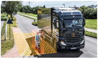
Continental's turn assist uses visual and acoustic signals to warn drivers of a possible collision.
